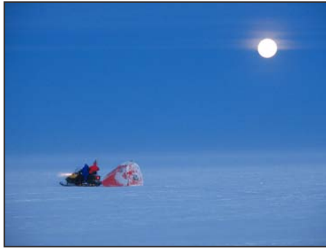
Summit science techs measure snow accumulation and tow a GPS unit to survey the surface elevation for correlation with ICESat, a study of ice-sheet topography.
