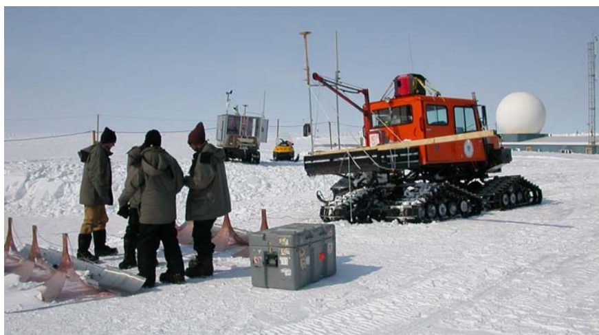
Four KU students connect radar antennas to a Tucker Sno-Cat (large orange tracked vehicle) that will then be used to drag the antennas over the ice and collect data. MARVIN is in the background. Photo: Dennis Sundermeyer
