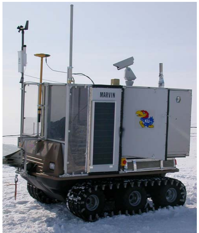
This prototype was created by modifying an all-terrain vehicle with a metal shell and adding various sensors and actuators to provide autonomous capability.
