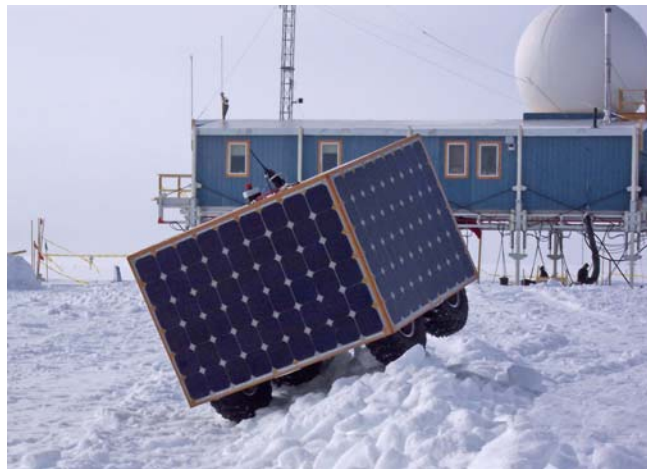
Designed to drive over rolling sastrugi on the Antarctic plateau, the robot demonstrates its capability to drive over wind-rows of plowed snow. Although it looks precarious, the robot has a very low center of gravity and plenty of torque for negotiating such obstacles.
